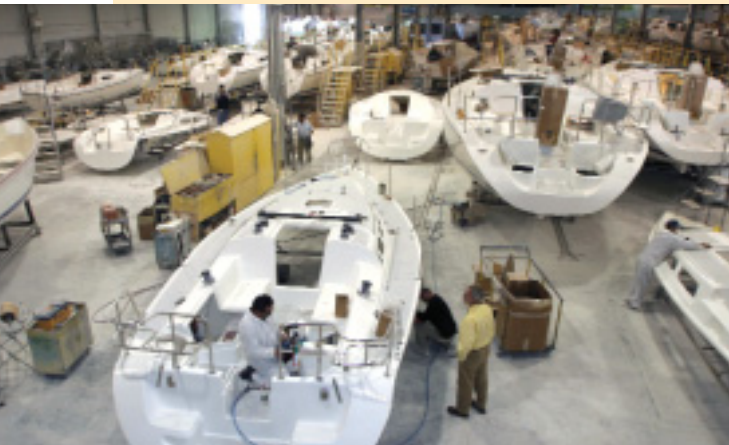
On models built in California, engine and interior components are passed below for installation into a completed shell of hull and deck. Obviously, those parts have to pass through one hatchway or another to get there, so they can also come back out for repairs when the time comes. Douglas (in yellow shirt) says it's a company goal to make a boat that is very repairable; all parts can be removed using hand tools and without disturbing other elements. The company makes an effort to sell replacement parts for all models, no matter how old, and Douglas touts Catalinas as good project boats for someone looking to rescue a fixer-upper. It would be cheaper to run plastic trim around the transom-hull joint, but the extra hours to create a seamless transition "are worth it for the look," Douglas says
