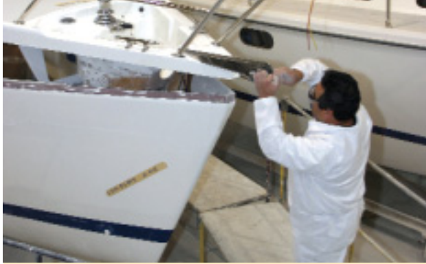
Catalina joins hull and deck early in the build process. Depending on the model, hull-to-deck joints are either overlapped external or internal flanges or outward-turning flanges
