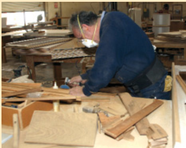
The wood mill turns out solid-wood surrounds, not veneer, for the door frames and furniture edges that take the most wear. All surfaces are clear-coated, not stained, so the color can be matched when refinished. All doors are mounted on piano hinges. Cabin soles in 2004 boats are a teak-and-holly-look-alike high-density laminate
