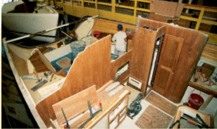
Catalina builds its 310, 350, 387, 400, and 470 models at its plant in Largo, Florida, where interiors are constructed in open hulls prior to the deck installation. Heads in Florida-built boats are built as modules and dropped into place whole. Large hatches still assure that all mechanical and interior parts are removable. Boats built on both coasts have bulkheads fixed with adhesives and fasteners to act as transverse diaphragms while carrying no rigging loads
